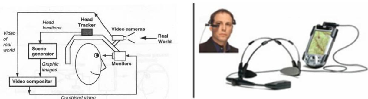
Figure 1.- Conceptual diagram of an Augmented Reality system
